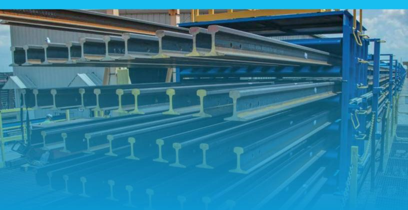
Holland has engineered and manufactured rail trains for ten years with a number of designs that can be applied to new, used, re-purposed, customer supplied and re-manufactured rail cars. They are designed to meet "B" or "C" railroad maintenance of way work envelope and RUM compatible.
